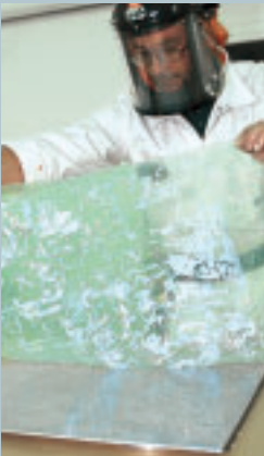
Special effects are created by applying and/or removing paint using film.
